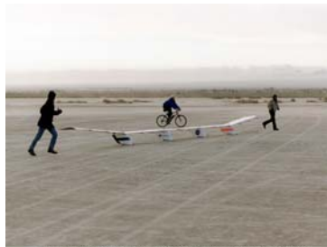
Dryden Flight Research Center EC97-43931-26 Photographed Feb1997 As crewmen jog or cycle alongside, a quarter-scale flying model of AeroVironment's Centurion flying wing rolls across a dry lakebed during pre-flight taxi tests. (NASA/Brent Wood)
